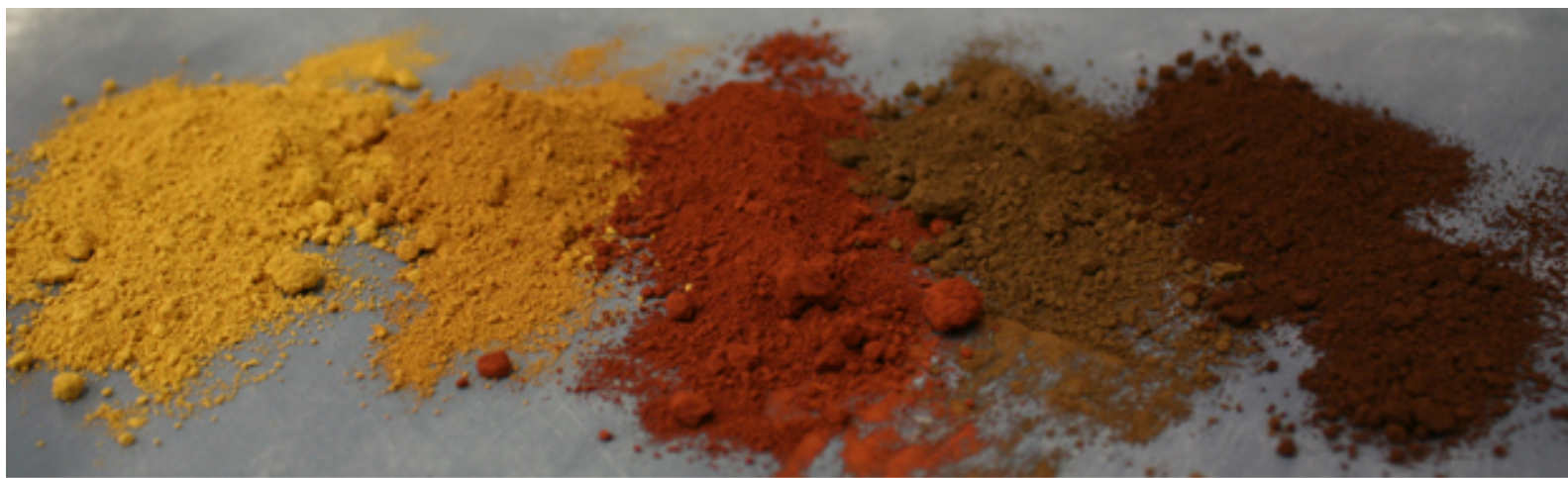
Natural Iron Oxides Dry Pigments: Yellow Ochre, Raw Sienna, Burnt Sienna, Raw Umber, and Burnt Umber
